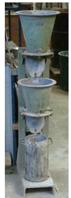
FigureNo.02 – Apparatus Used to Conduct the Compacting Factor Test
