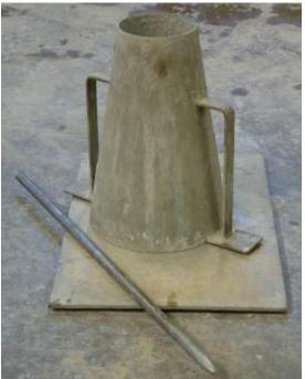
Figure No. 01 – Equipment Required to Conduct a Slump Test
